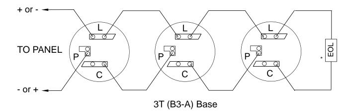
\* EOL: End of Line devices usually come with the fire alarm control panels or other devices to which the detectors connect.
